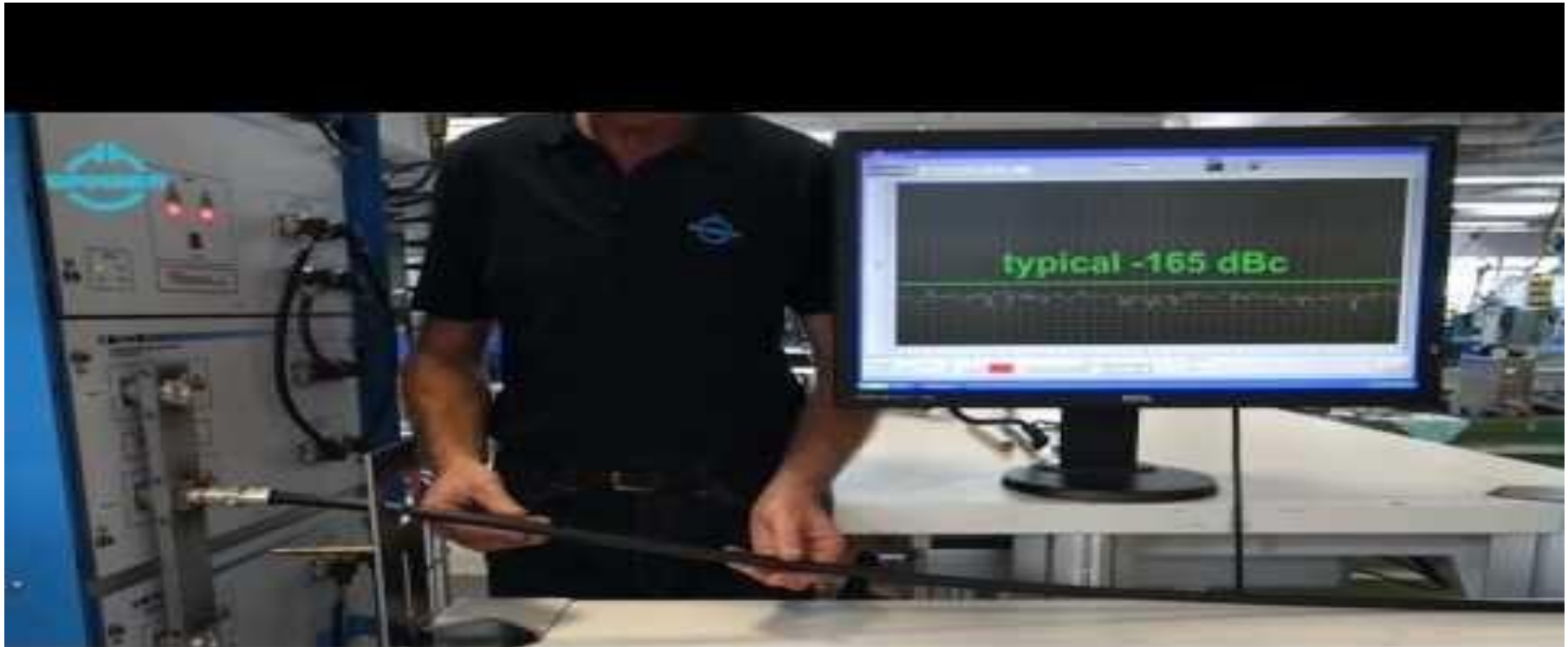
Test of SF1/2" Jumper with 4.3-10 Male Hand Screw JS12-43MH43MS-2M; -160 dBc max.; -165 dBc typ.
